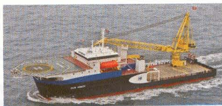
The high block coefficient hull is optimised for stationkeeping
