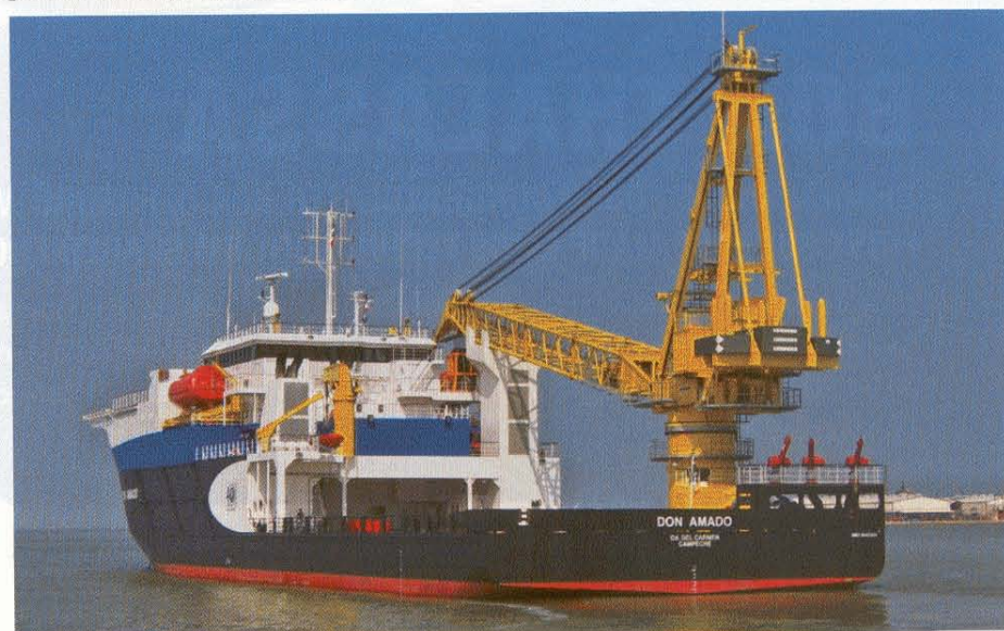
Don Amado has a reduced draught, which enables the ship to work into and out of smaller Mexican ports and harbours
