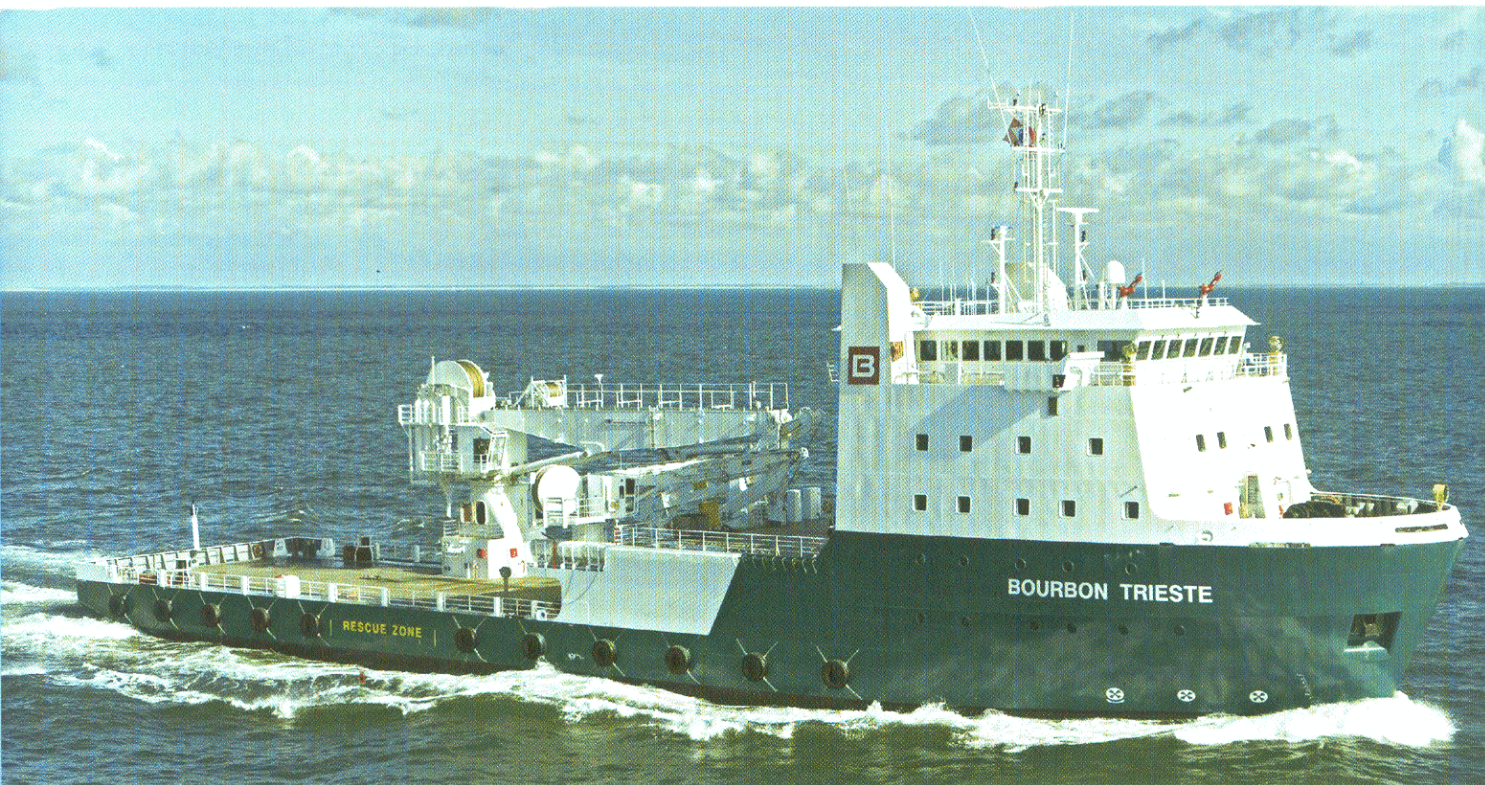
De Hoop also constructed one of Groupe Bourbon's latest newbuilds, Bourbon Trieste an 82m long vessel of DP2 class
