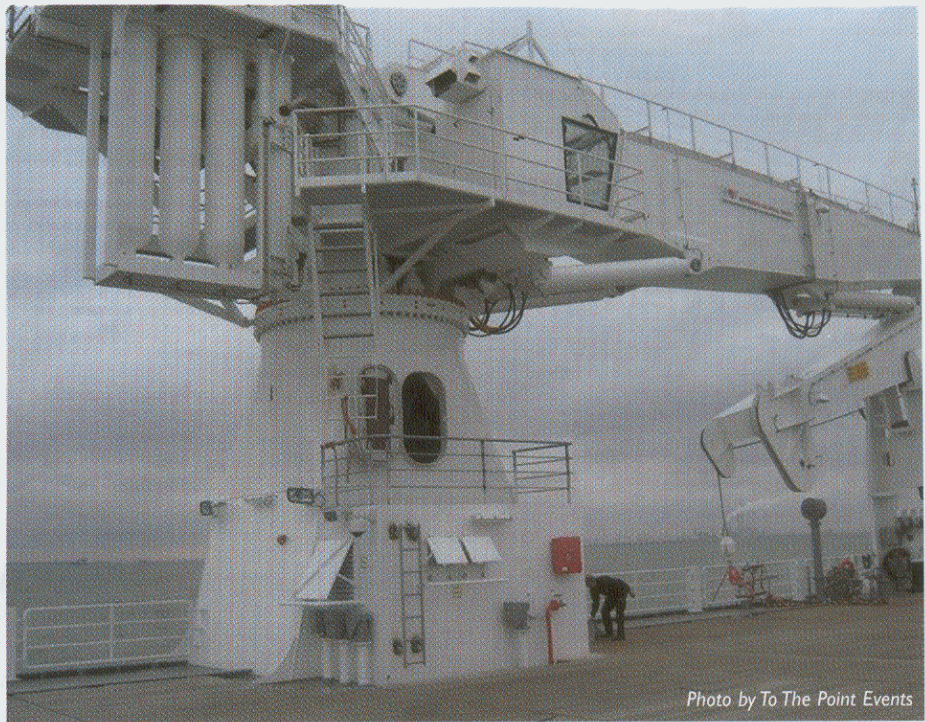
The knuckle-boom crane has active heave compensation
